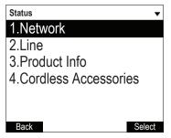
c. On the Status menu, ensure that **Network** is highlighted, and then press **SELECT**. The Network screen appears.
